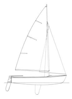
The FJ is a high performance, two person sailboat used in our Level 3 class and frequently in collegiate racing programs. An FJ has two sails: a mainsail and a jib. With flotation compartments, FJs don't sink and can be used in capsizing drills for older students. Our FJs are usually kept on dollies south of the swimming beach or on the grass near the beach when not being used.
