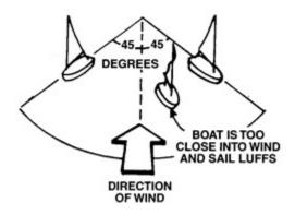
The angle that a boat cannot produce power to move is known as the no go zone.
