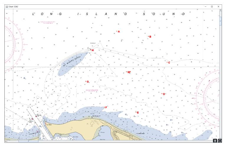
Circle is aligned on Magnetic North, and is 1 NM in diameter.
