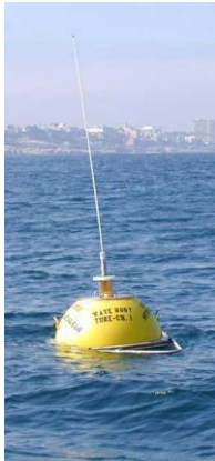
Weather buoy 46221 Santa Monica Bay Y”28” FL (5)Y20S (SMB)
