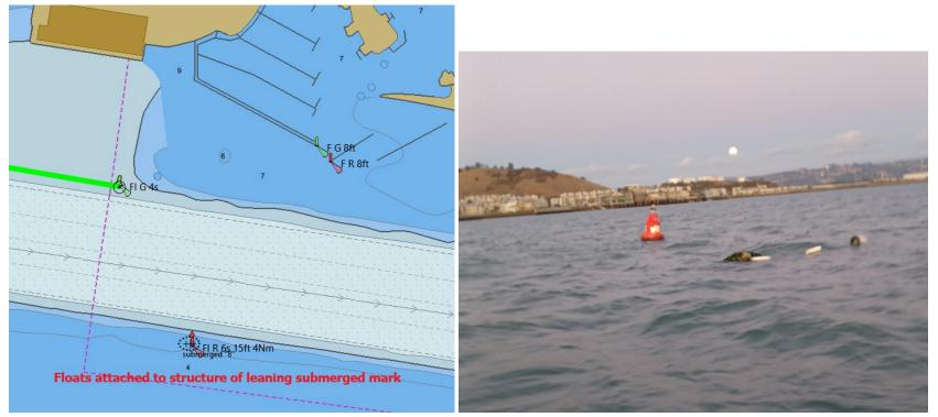
**Remains of ferry landing demolition:** There are two snags which are visible at about a -1.0ft tide. They are marked by orange floats. The northeastern corner of a sunken barge is marked with a dock bumper closer in towards the remaining part of the landing.
