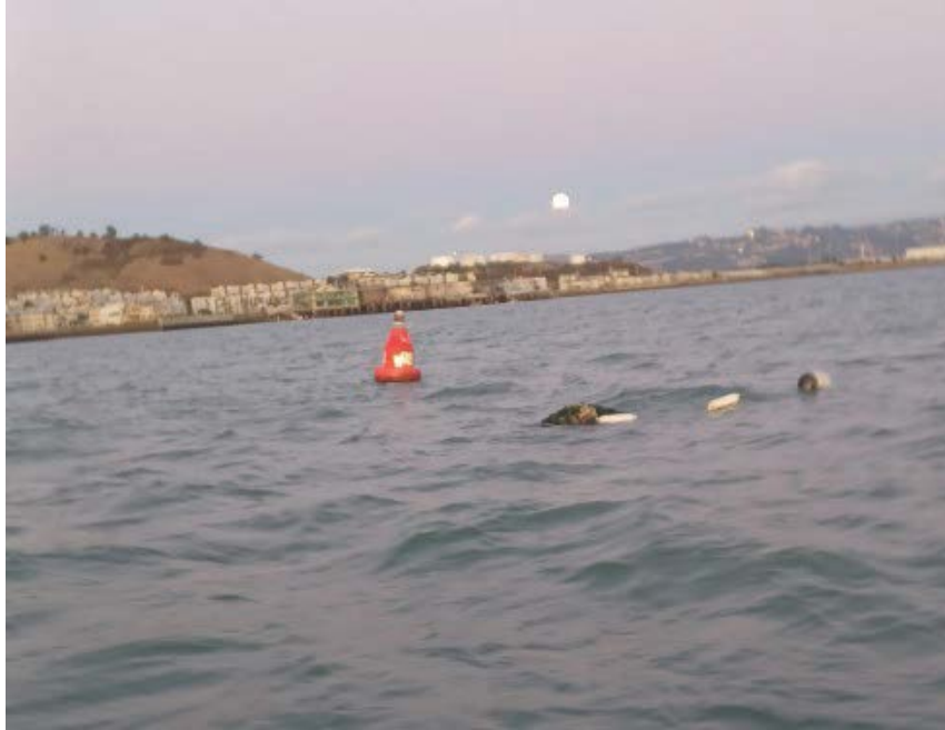
Richmond sewage outfall pipe markers: "2" has no light and can be submerged during high tide and strong currents (still exists): The photo was taken at a 6.8ft tide, 0.8kt current. You can see "1" in the background.
