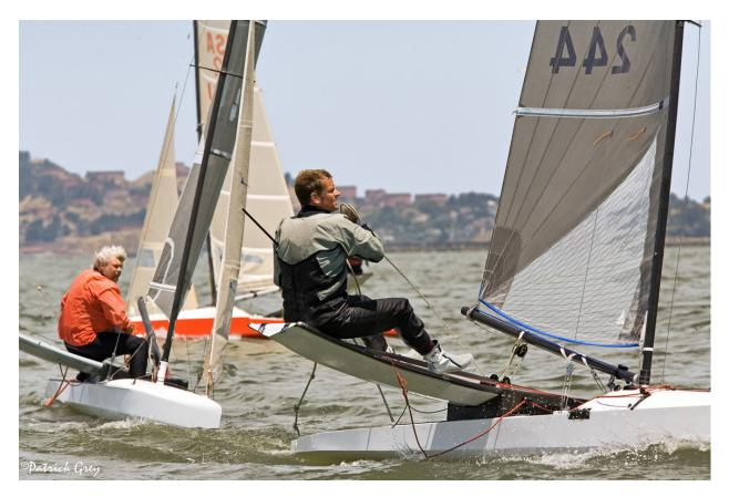
A one-design class from 1971 to 2008, the International Canoe officially became a developmental class in 2009, operating under a simple set of rules that define the hull's allowable length (4900-5200mm) and minimum beam and the boat's overall minimum weight excluding sails. The total allowable sail area is 10 square meters. The
